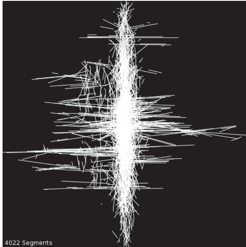
FIG. 3.9. Density-based clustering (unconstrained data). For unconstrained data sets, the density-based approach had difficulty growing a cohesive trajectory through the data set.
